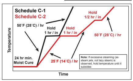
to spalls/explosions at elevated furnace temperatures. This is of special concern in floors/hearths.
