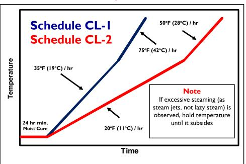
**CAUTION / WARNING**This schedule assumes that heating for bake out is regulated and is applied in a controlled, uniform manner. Note that the target control temperatures are to be measured by thermo-
