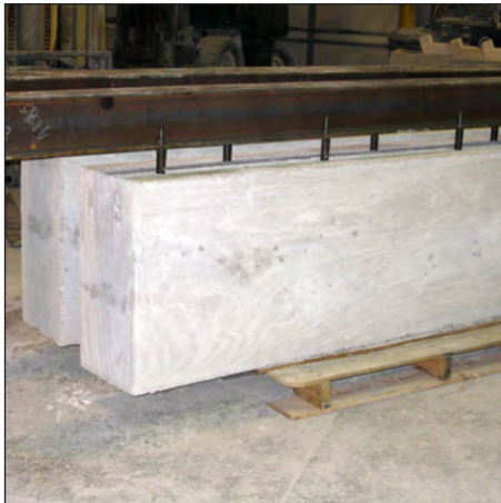
Sills and Lintels
