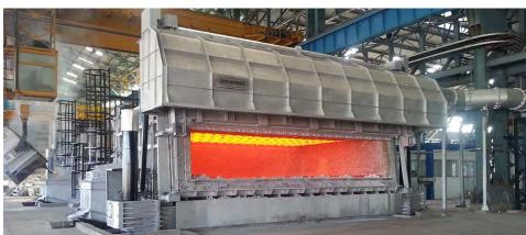
For aluminum processors, one of the costliest operational challenges in high-production environments is the aggressive formation of corundum deposits in furnaces. Excessive, damaging, and costly, corundum growth can be mitigated with the right refractory materials, coupled with proper maintenance.
