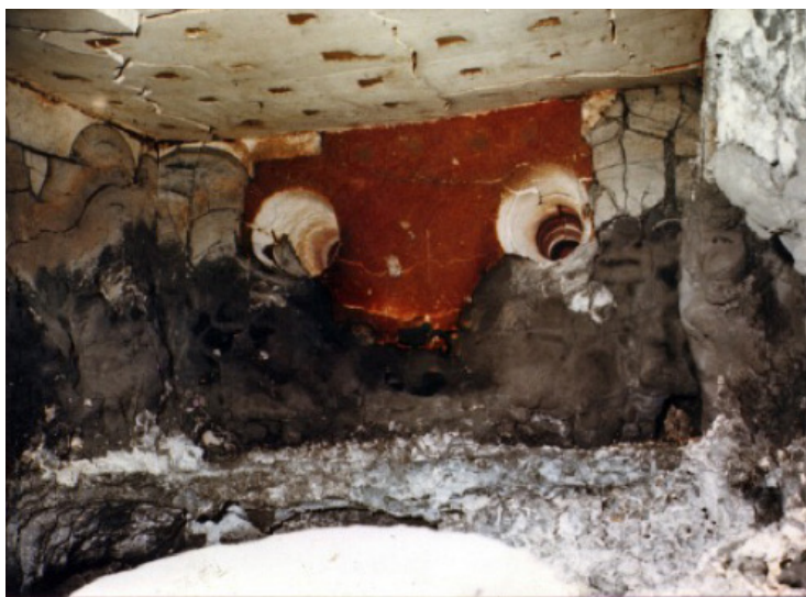
Corundum under heat expansion cracks the refractory.
