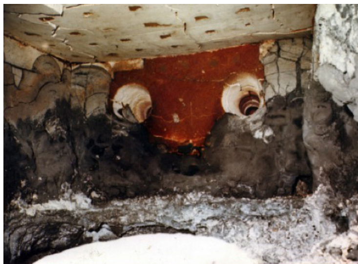
Corundum under heat expansion cracks the refractory.
